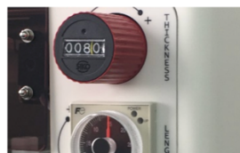
turn the dials for setting and adjusting the size or volume of rice sheets.
